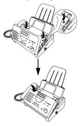
Reinsert the paper in the paper tray and push the paper release plate back down
